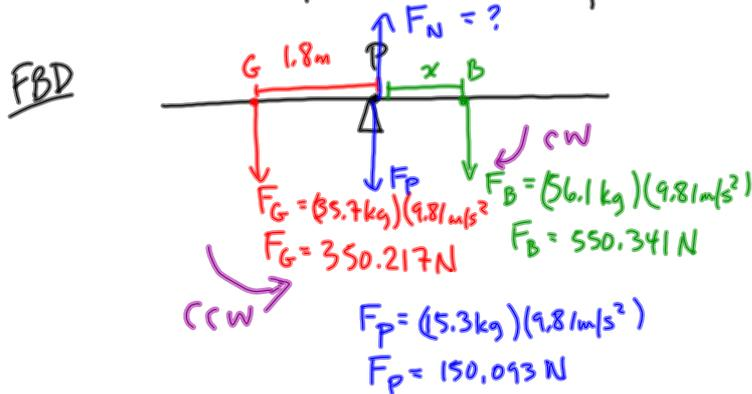
a) For there to be static equilibrium, the net torque on the teeter-totter must be ZERO!
